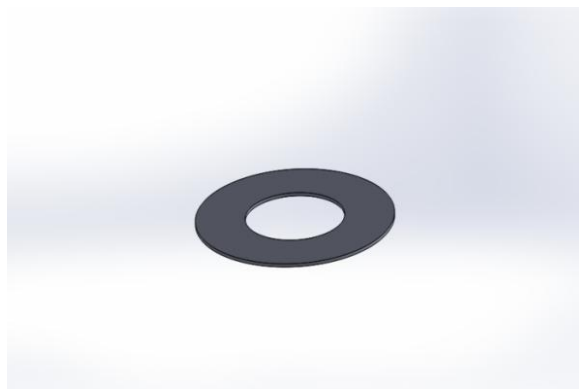
Fig. 4. SolidWorks 2014 illustration of Flat Rigid-ring Baffle of 0.1 m width [31]
