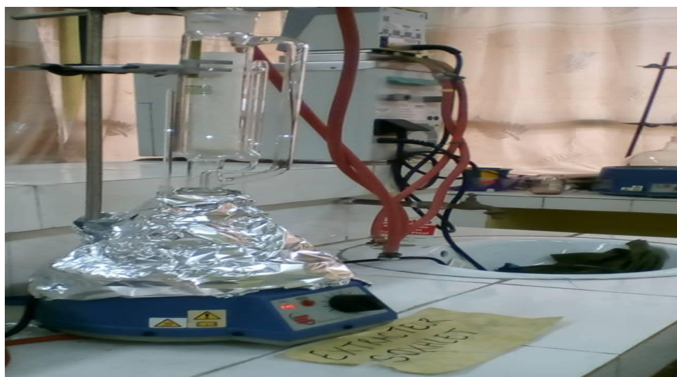
Fig. 1b. Soxhlet extraction setting used
