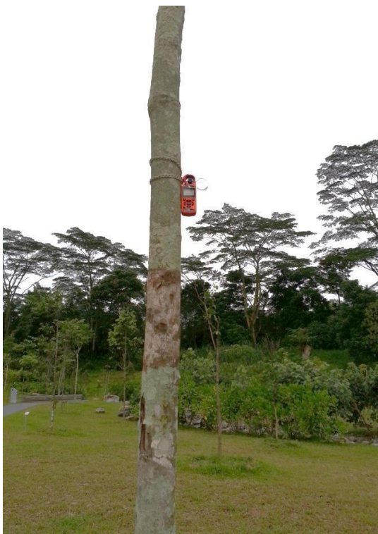
Fig. 8. Instrument mounted on a tree at screen height of 2m above ground at Clean Tech Park
