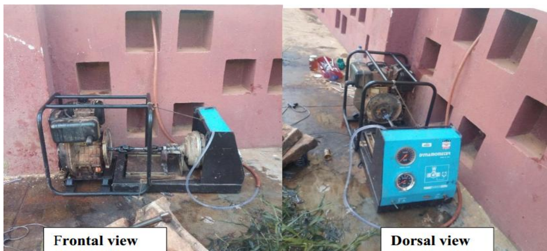
Fig. 4. Dynamometer connected to the diesel engine
