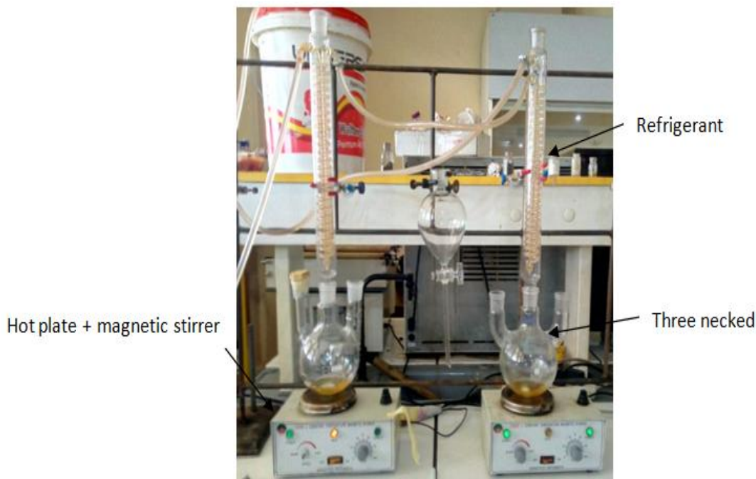
Fig. 1. Experimental device for transesterification reactions
